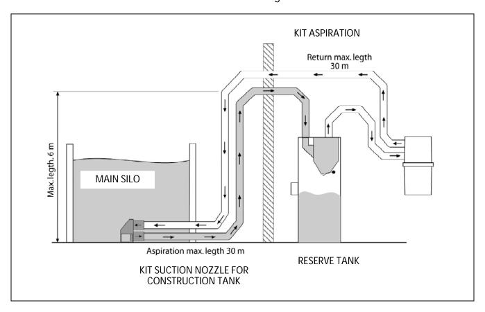
**IMPORTANT:** At each end of the pellet suction and air return hose, the copper cables must be connected to the earth connection terminals provided for this purpose.
